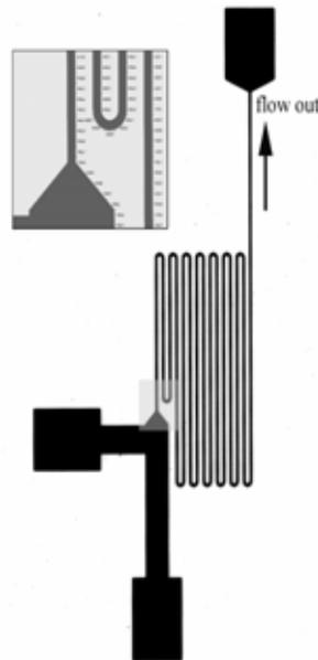
**Figure .2.** Schematic of 14 cm long flow chamber. Channel is 100  $\mu$ m wide.
