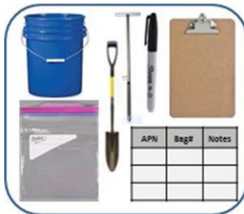
Figure 1. Materials needed for soil sampling.
