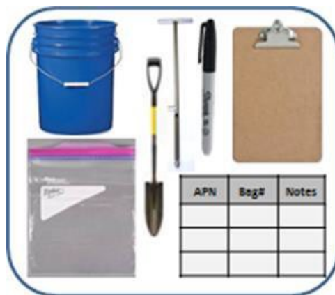
Figure 1. Materials needed for soil sampling.
