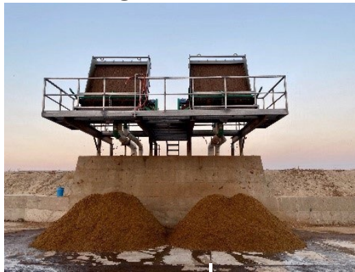
(Left – Compost Bedded Pack Barn with a recently tilled loafing area installed for a 2017 AMMP project. / Middle - Kooistra 2022 AMMP Recipient Manure solid-liquid separator / Right - Windrows for composting separated manure solids at a 2019 AMMP project)
