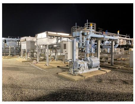
**Image 24.** Upgrader equipment at the CalBioGas West Visalia Cluster, which receives biogas from S&S Dairy.
