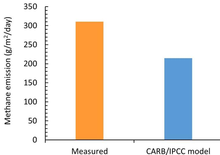
Figure 85. Measured and modeled methane emissions from the settling basin on the Foxtrot dairy on October 15.
