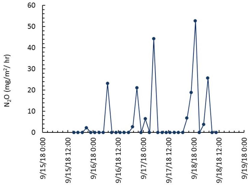
Figure 45. Emission rates of N<sub>2</sub>O from the lagoon on the Bravo dairy.
