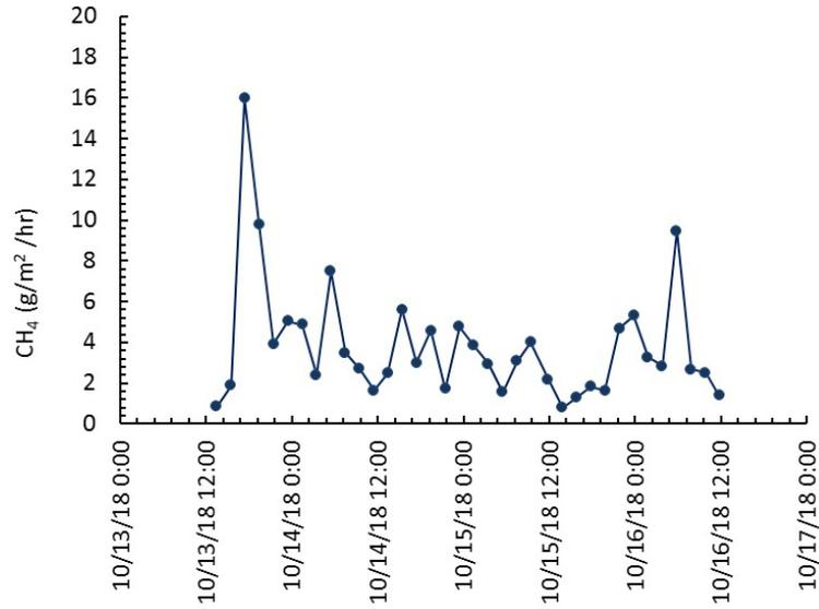
**Figure 71. Emission rates of CH<sub>4</sub> from the lagoon in the Foxtrot dairy.**
