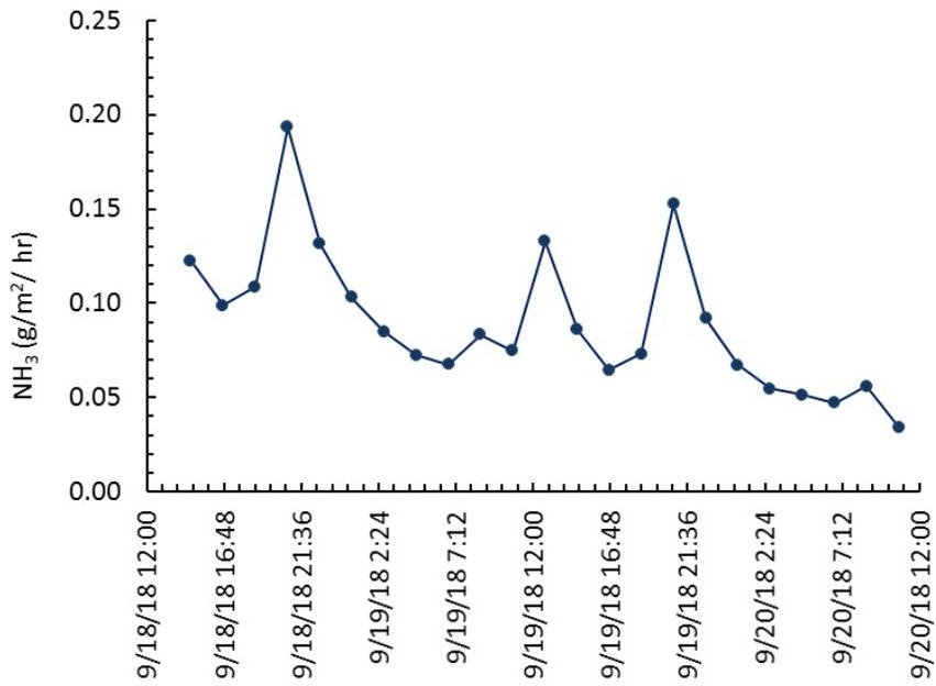
Figure 40. Emission rates of NH<sub>3</sub> from the settling basin on the Bravo dairy.
