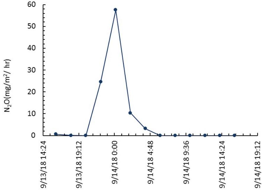
Figure 33. Emission rates of N<sub>2</sub>O from the settling basin on the Alpha dairy.
