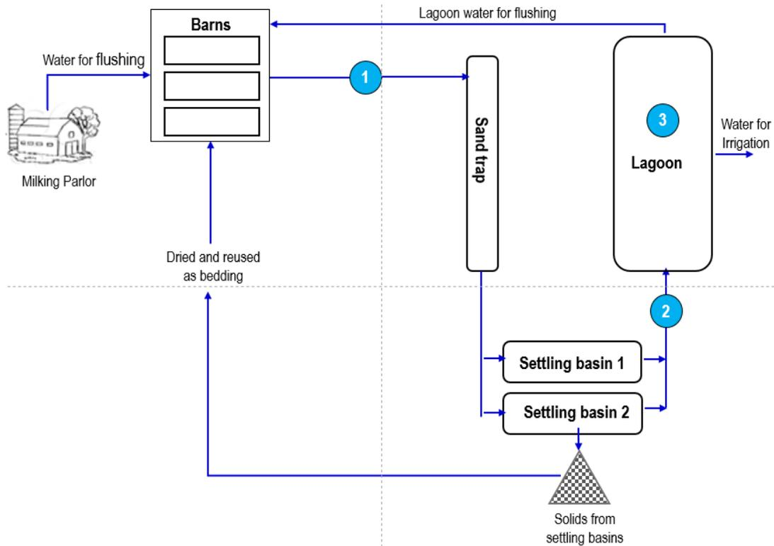
**Figure 18. Single-line flow diagram for the manure management system on Alpha dairy.**
