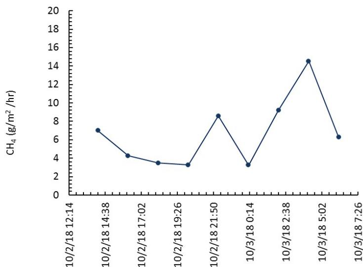
Figure 51. Emission rates of CH<sub>4</sub> from the settling basin in the Delta dairy.
