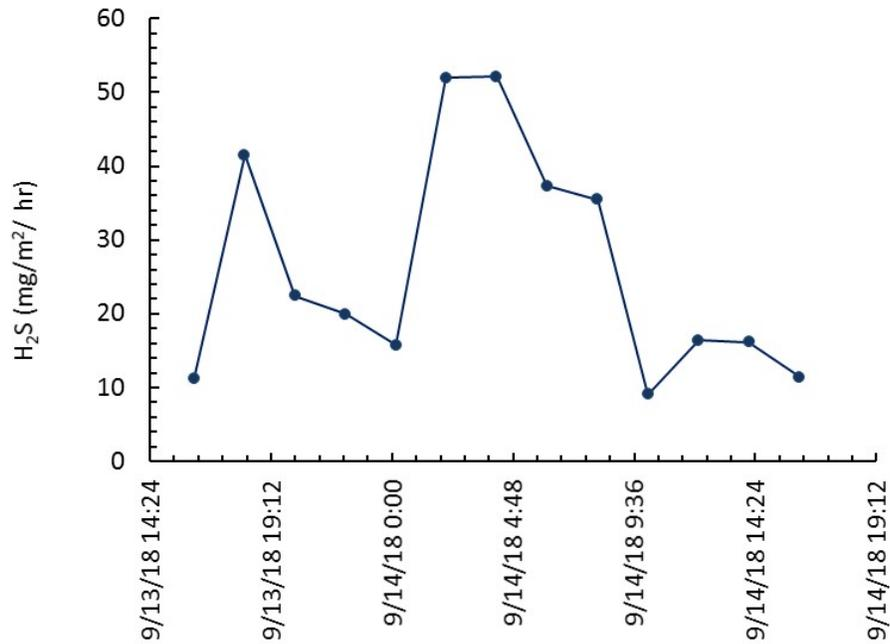
Figure 34. Emission rates of H<sub>2</sub>S from the settling basin on the Alpha dairy.
