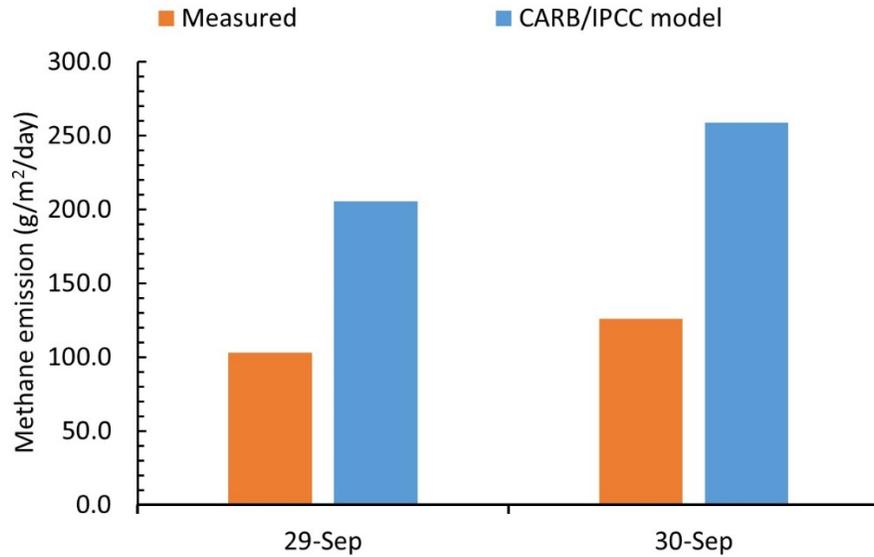
**Figure 80. Measured and modeled methane emissions from the lagoon on the Delta dairy.**
