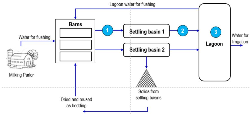
Figure 19. Single-line flow diagram for the manure management system on Bravo dairy.
