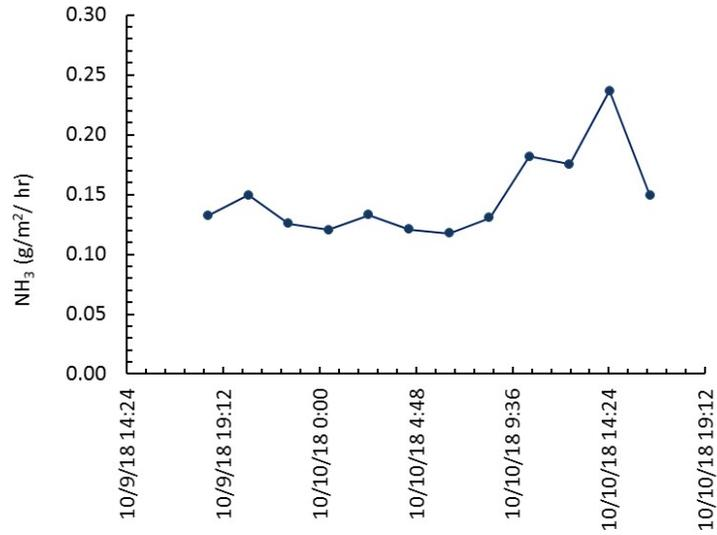
**Figure 60. Emission rates of NH<sub>3</sub> from the settling basin on the Echo dairy.**
