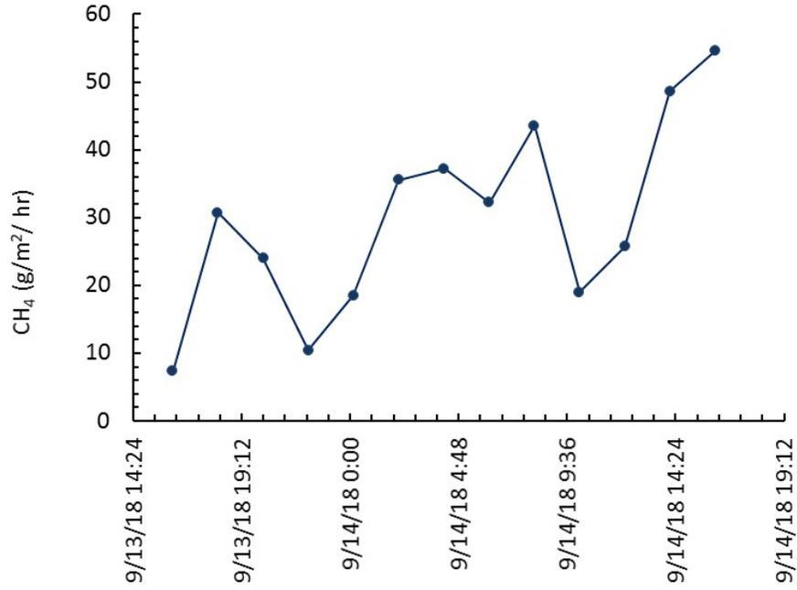
Figure 31. Emission rates of CH<sub>4</sub> from the settling basin on the Alpha dairy.
