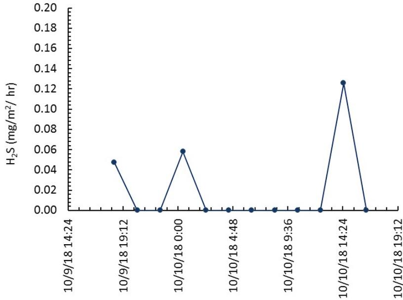
**Figure 62. Emission rates of H<sub>2</sub>S from the settling basin on the Echo dairy.**
