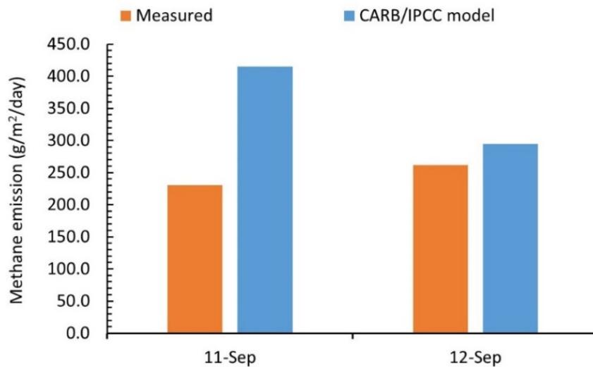
Figure 75. Measured and modeled methane emissions from the lagoon on the Alpha dairy.
