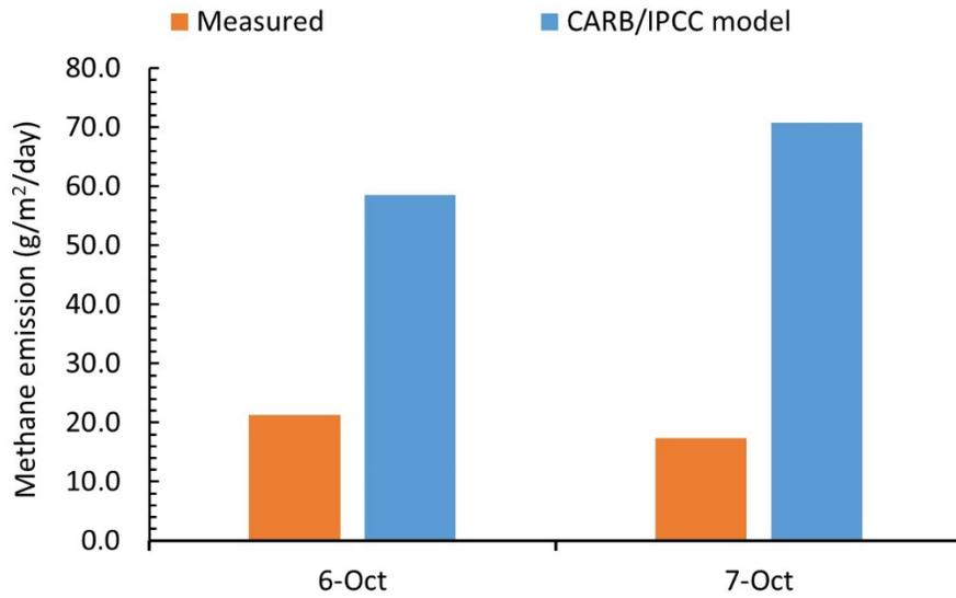
**Figure 82. Measured and modeled methane emissions from the lagoon on Echo dairy.**
