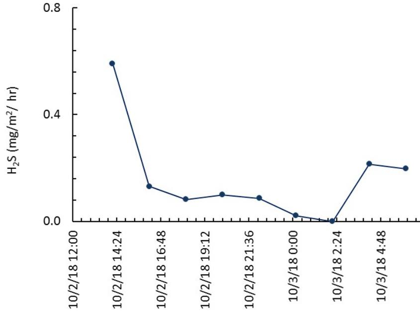
**Figure 54. Emission rates of H<sub>2</sub>S from the settling basin on the Delta dairy.**
