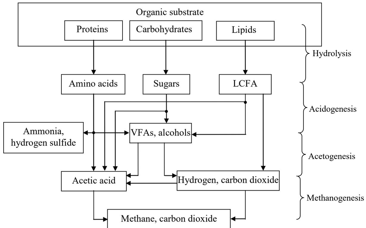
**Figure 1. Main sub-processes involved in anaerobic digestion process (adapted from Pavlostathis and Giraldo-Gomez, 1991; Batstone et al., 2002).**
