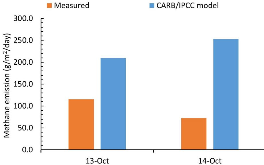
Figure 84. Measured and modeled methane emissions from the lagoon on the Foxtrot dairy.
