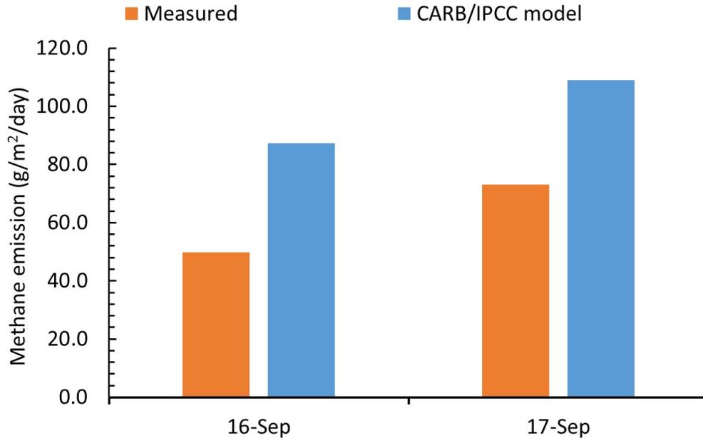
Figure 77. Measured and modeled methane emissions from the lagoon on the Bravo dairy.
