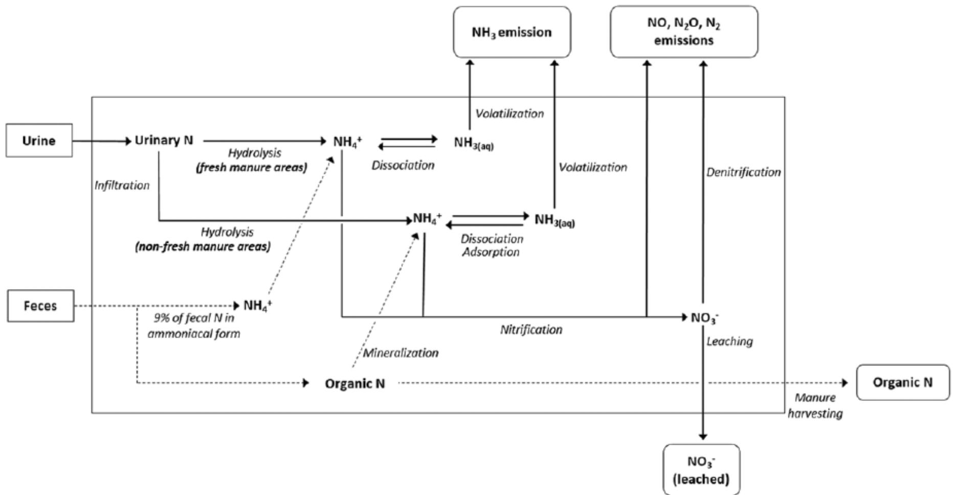
Figure 2. Nitrogen flow through processes as simulated for open lots (Bonifacio et al., 2015)
