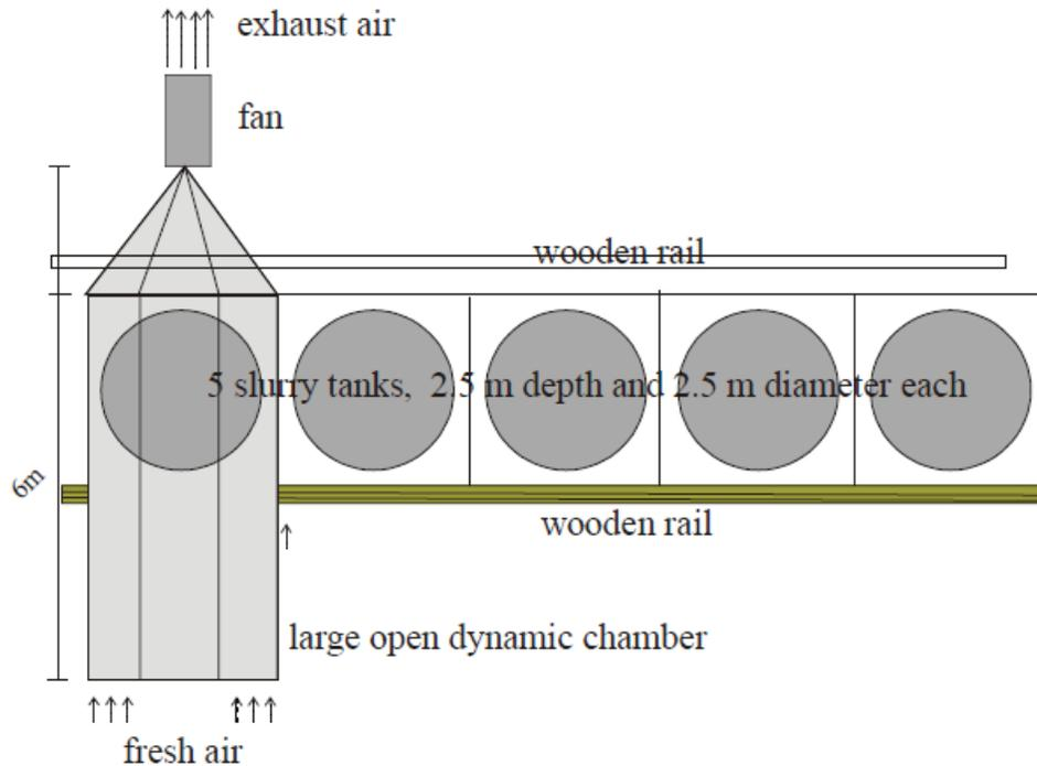
**Figure 14. Open dynamic chamber moving over wooden rails (Amon et al., 2006).**
