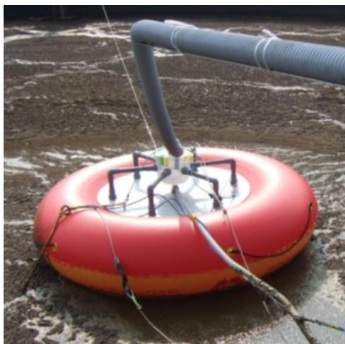
**Figure 17. A floating open chamber on the storage tank surface (Minato et al., 2013).**
