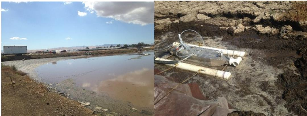
**Figure 29. The wind tunnel during the emission measurements from the lagoon (left) and the settling basin (right) on Echo dairy.**
