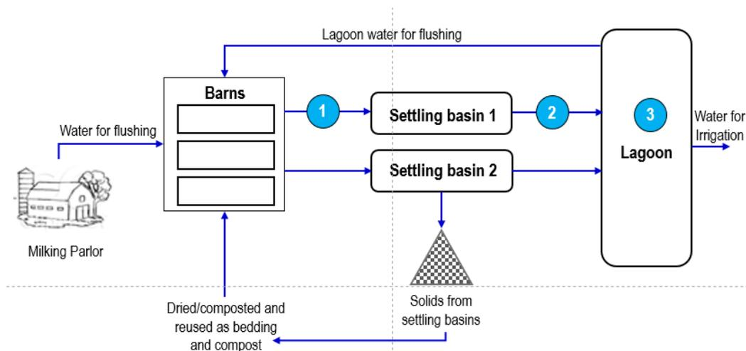
Figure 21. Single-line flow diagram for the manure management system on Delta dairy.
