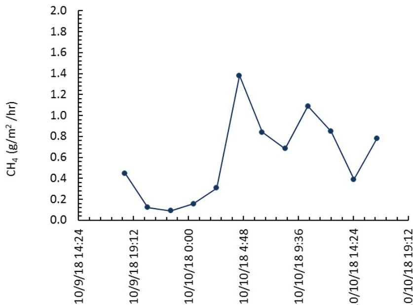
**Figure 59. Emission rates of CH<sub>4</sub> from the settling basin on the Echo dairy.**
