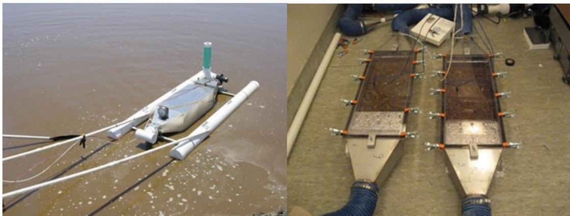
**Figure 12. A floating wind tunnel for measuring the emissions from lagoons (left); a wind tunnel used for measuring the emissions from slurry (right).**
