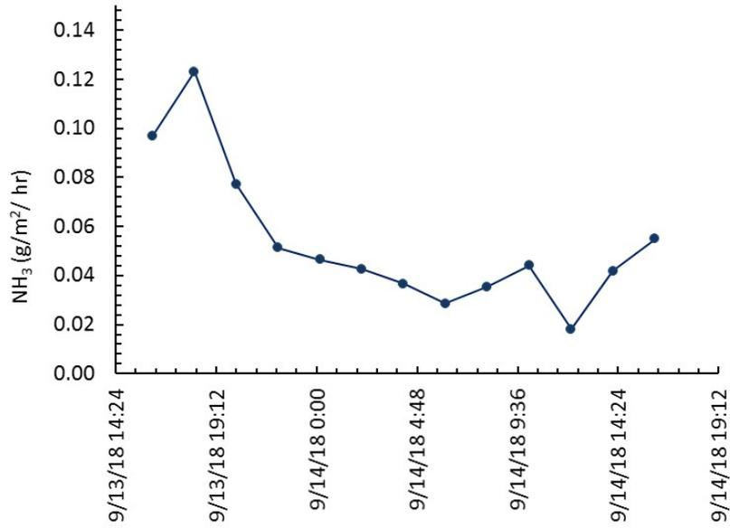
Figure 32. Emission rates of NH<sub>3</sub> from the settling basin on the Alpha dairy.
