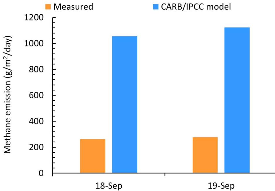
Figure 78. Measured and modeled methane emissions from the settling basin on Bravo dairy.
