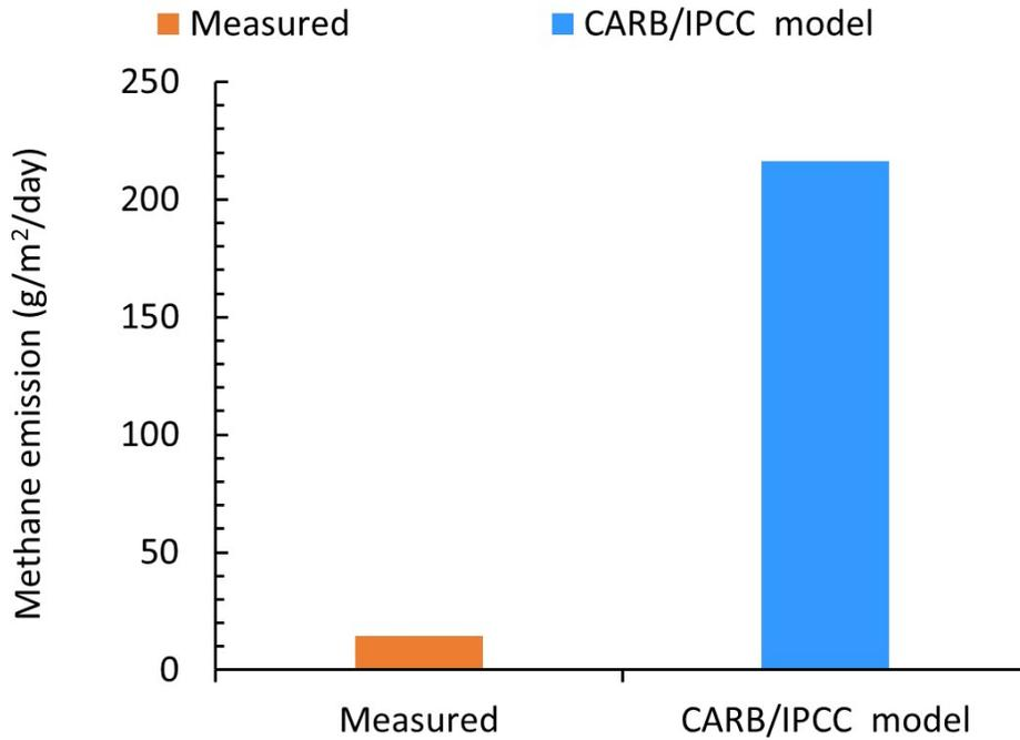
**Figure 83. Measured and modeled methane emissions from the settling basin on Echo dairy on October 8, 2018.**
