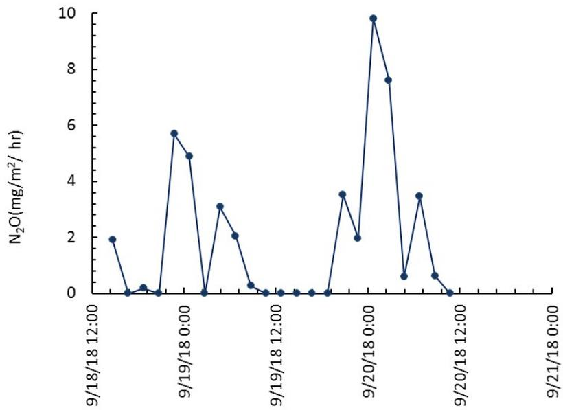
**Figure 41. Emission rates of N<sub>2</sub>O from the settling basin on the Bravo dairy.**
