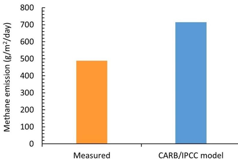
**Figure 76. Measured and modeled methane emissions from the settling basin on the Alpha dairy on September 13, 2018.**
