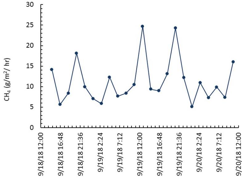
Figure 39. Emission rates of CH<sub>4</sub> from the settling basin on the Bravo dairy.
