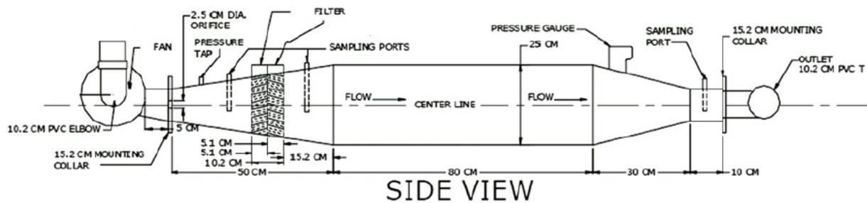
**Figure 26. Main parts and dimensions of the wind tunnel (adapted from Kumar et al., 2011).**
