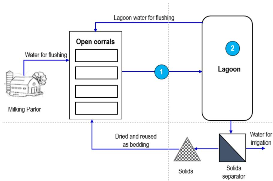
Figure 20. Single-line flow diagram for the manure management system on Charlie dairy.
