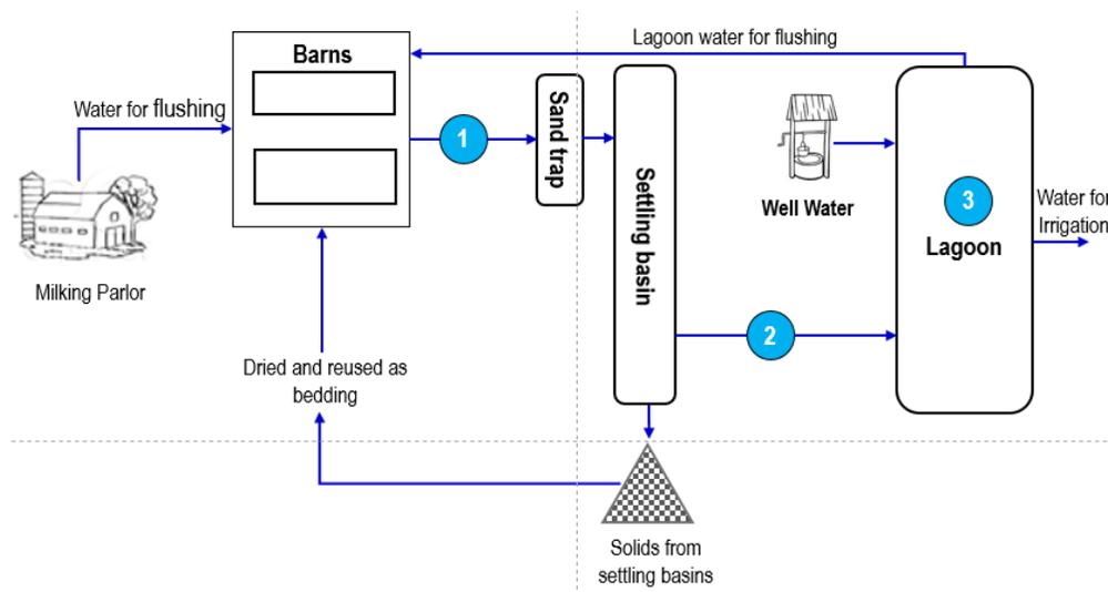
**Figure 22. Single-line flow diagram for the manure management system on Echo dairy.**
