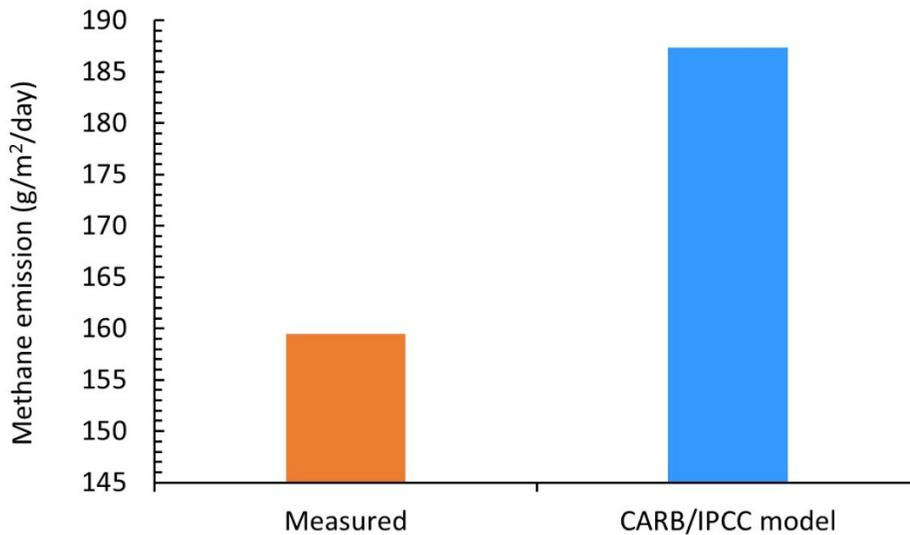
**Figure 81. Measured and modeled methane emissions from the settling basin on the Delta dairy on October 1, 2018.**
