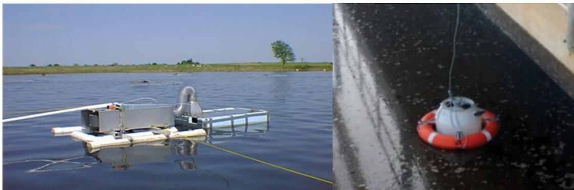
**Figure 15. A floating emission chamber (Heber et al., 2002), left; floating flux chamber used at a sewage treatment plant (Day et al., 2016), right.**
