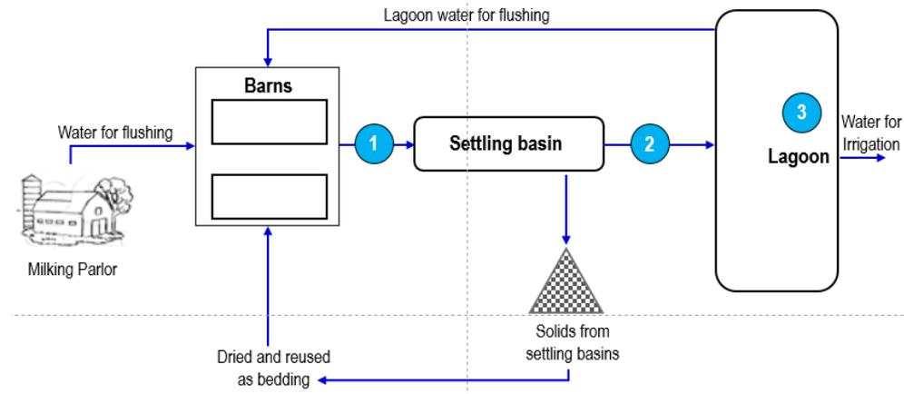
**Figure 23. Single-line flow diagram for the manure management system on Foxtrot dairy.**
