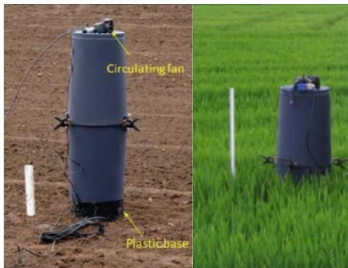
**Figure 16. Flux chamber used at rice fields (Day et al., 2016).**
