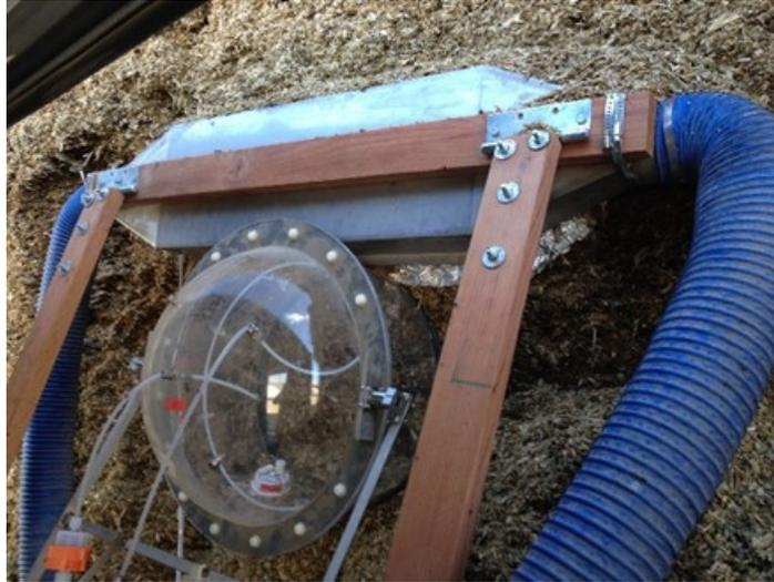
**Figure 13. Flux chamber and wind tunnel during measuring the emissions from a silage pile.**
