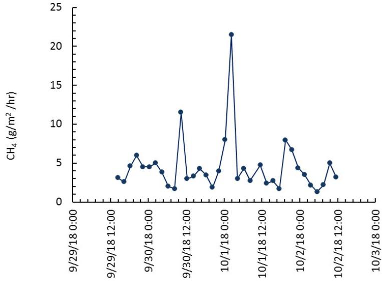
Figure 55. Emission rates of CH<sub>4</sub> from the lagoon on the Delta dairy.
