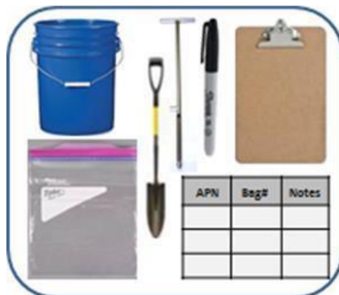
Figure 1. Materials needed for soil sampling.
