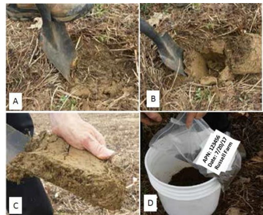
Figure 4. Taking samples with a shovel.
