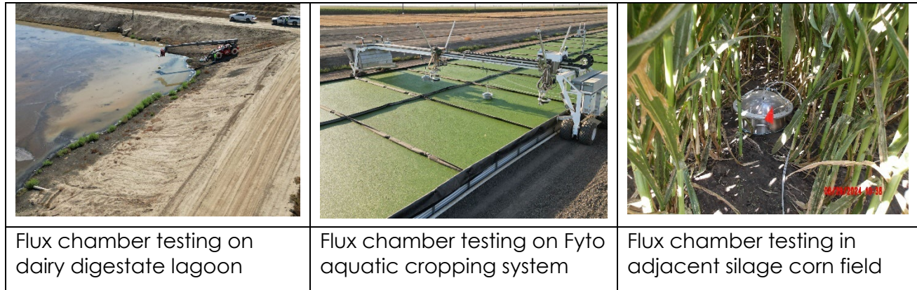
Figure 8: Direct gaseous emissions measurements were conducted by CE Schmidt at Rancho Teresita
