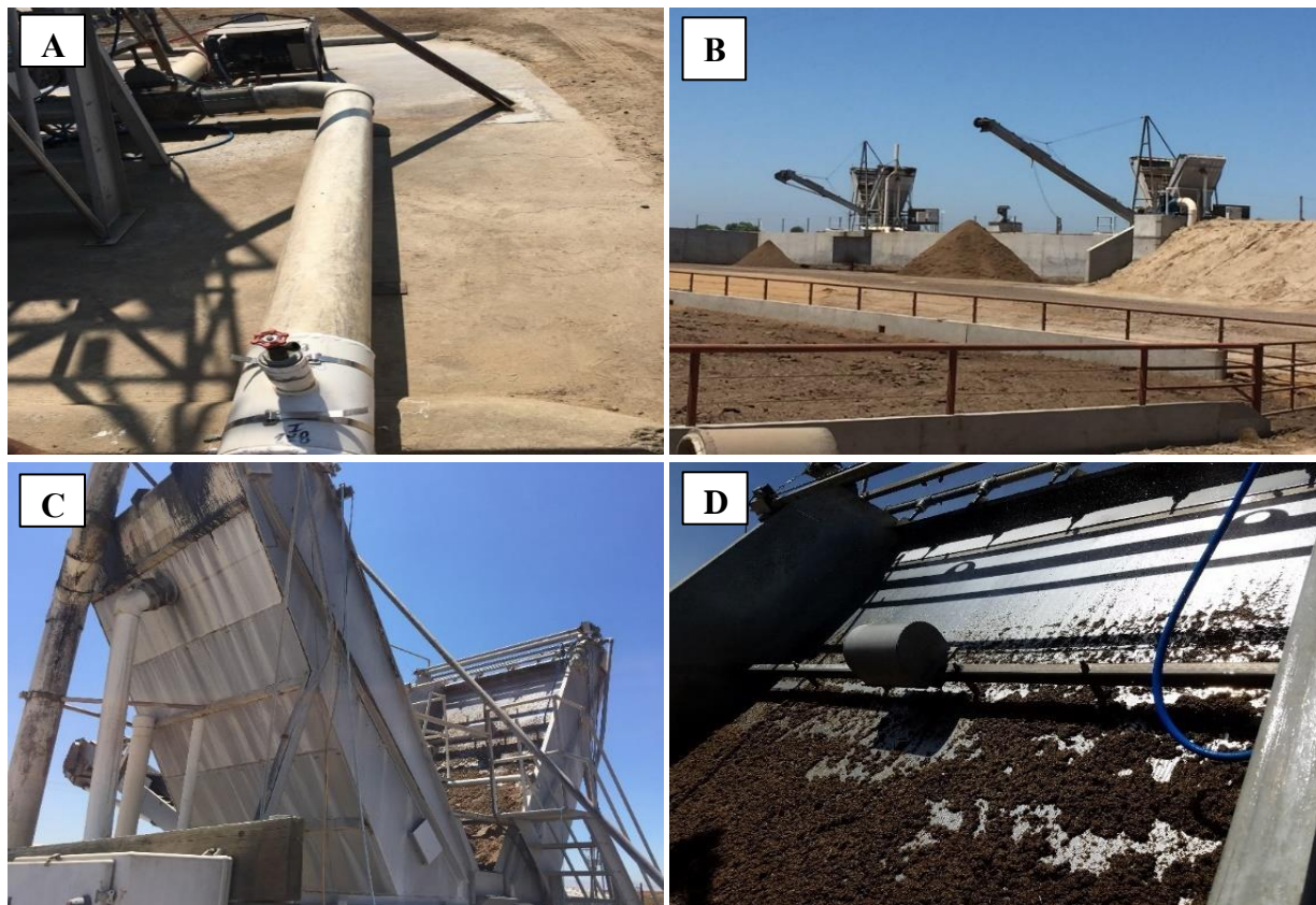
Figure 22. Dairy B: (A) flow meter installed on coarse separator inlet, (B) two mechanical separators, (C) coarse separator, and (D) flush manure flowing over separator screen
