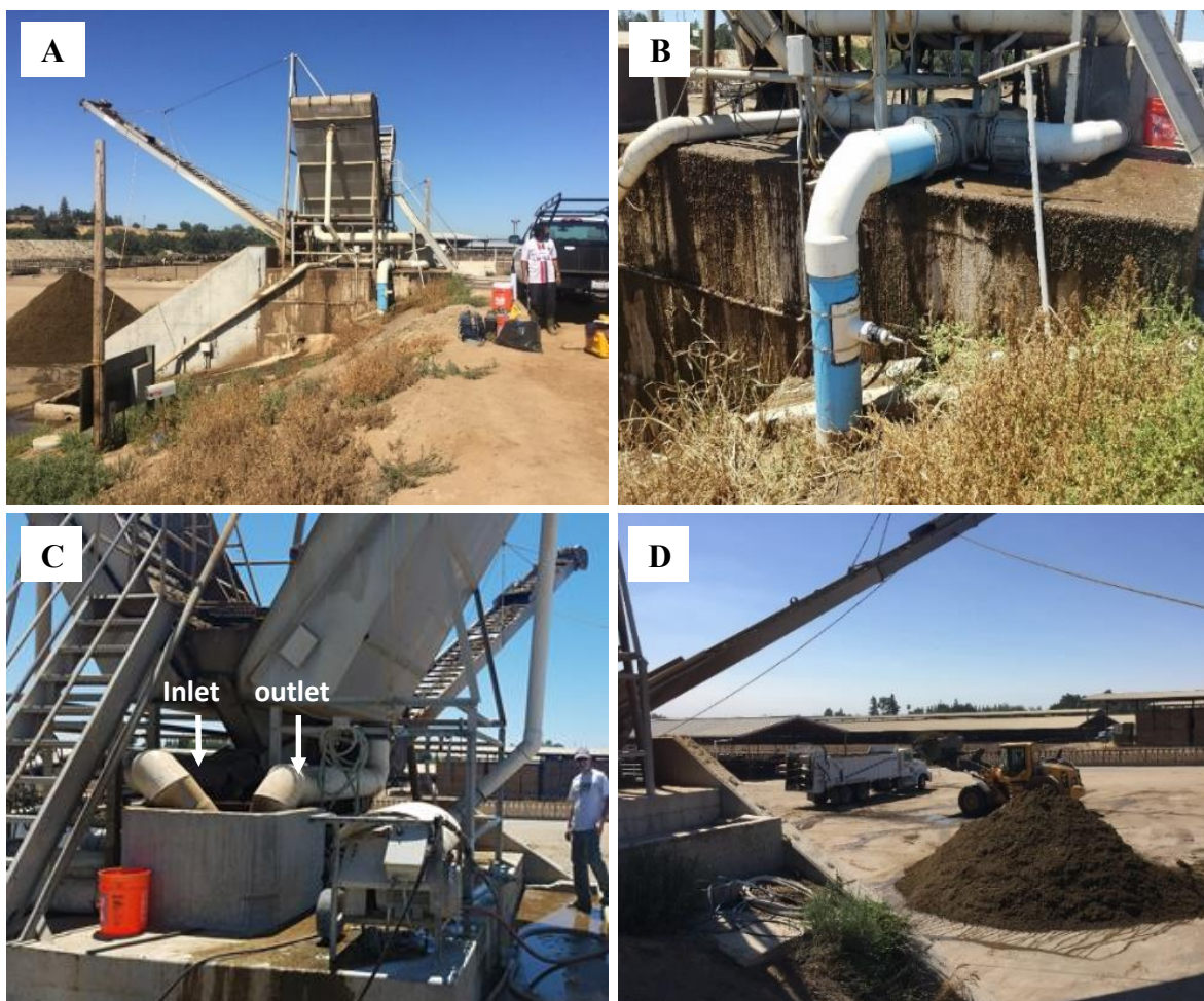
Figure 14. Dairy A: (A) separator, (B) inlet pipe and flow meter, (C) inlet/outlet sampling points, and (D) solids pile under the separator
