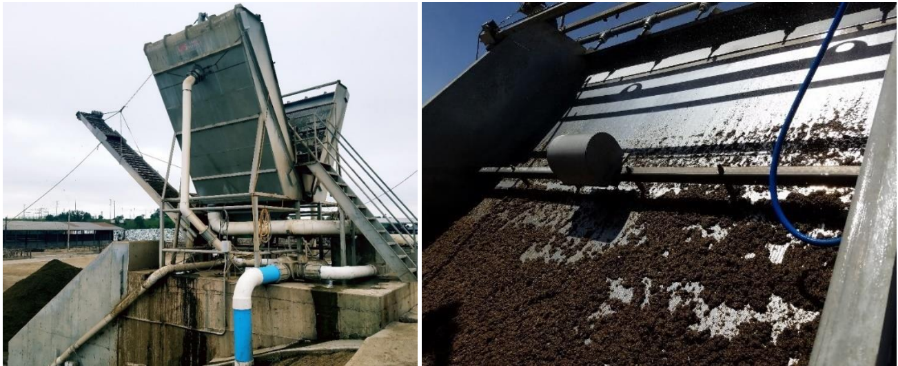
Figure 1. Dairy A: (Left) 1-stage sloped dual-screen separator, and (Right) closer view of the type of separator screen on Dairy's A and B
