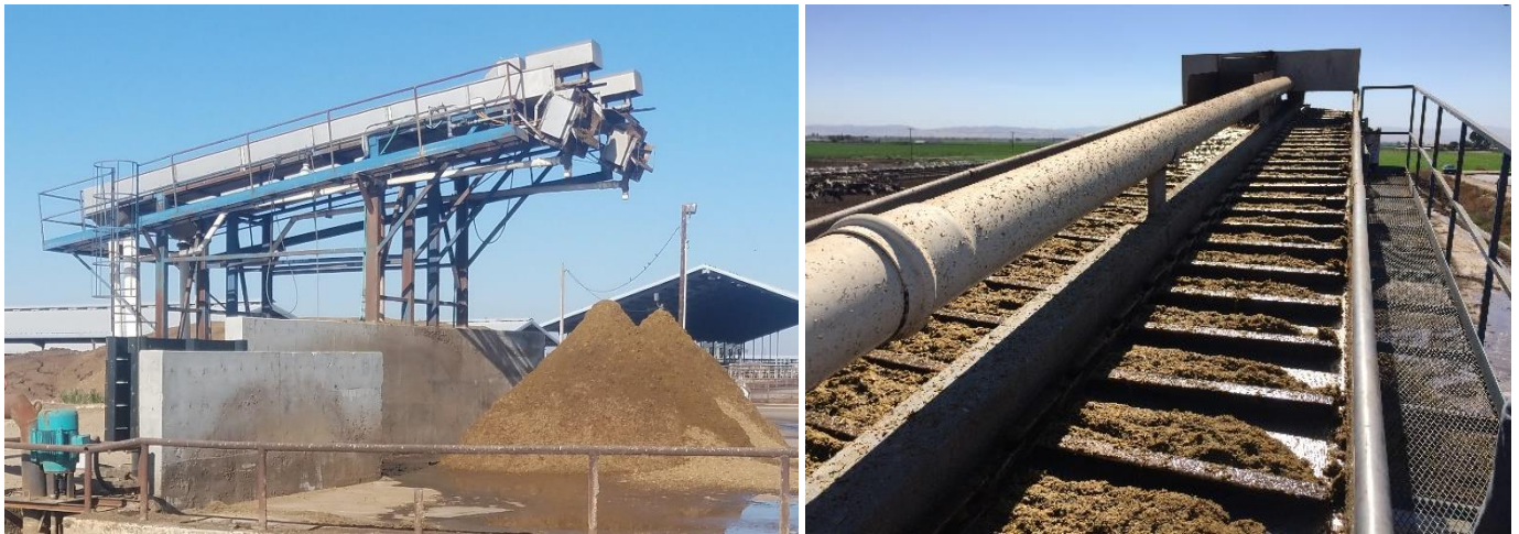
Figure 4. Dairy D: (Left) horizontal scraped-screen separator as seen from the ground and (Right) close up view of separator paddles and screen
