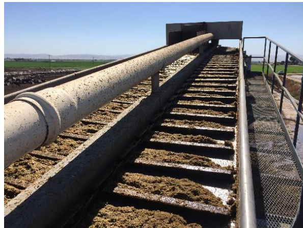
Figure 46. Dairy D*: Scraped screen separator in action
