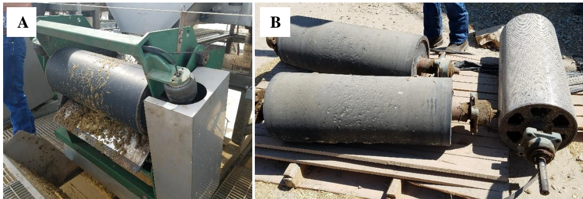
Figure 33. Dairy C: (A) Rotary drum separator, and (B) Separator roller press and rotary drum
