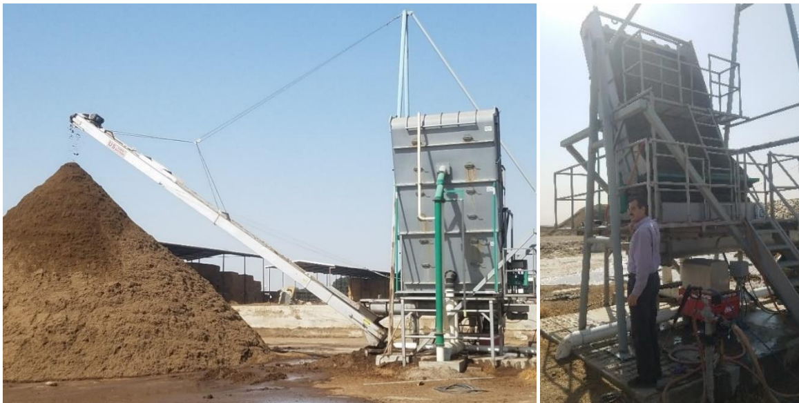
Figure 7. Dairy F: 1-stage sloped single-screen separator
