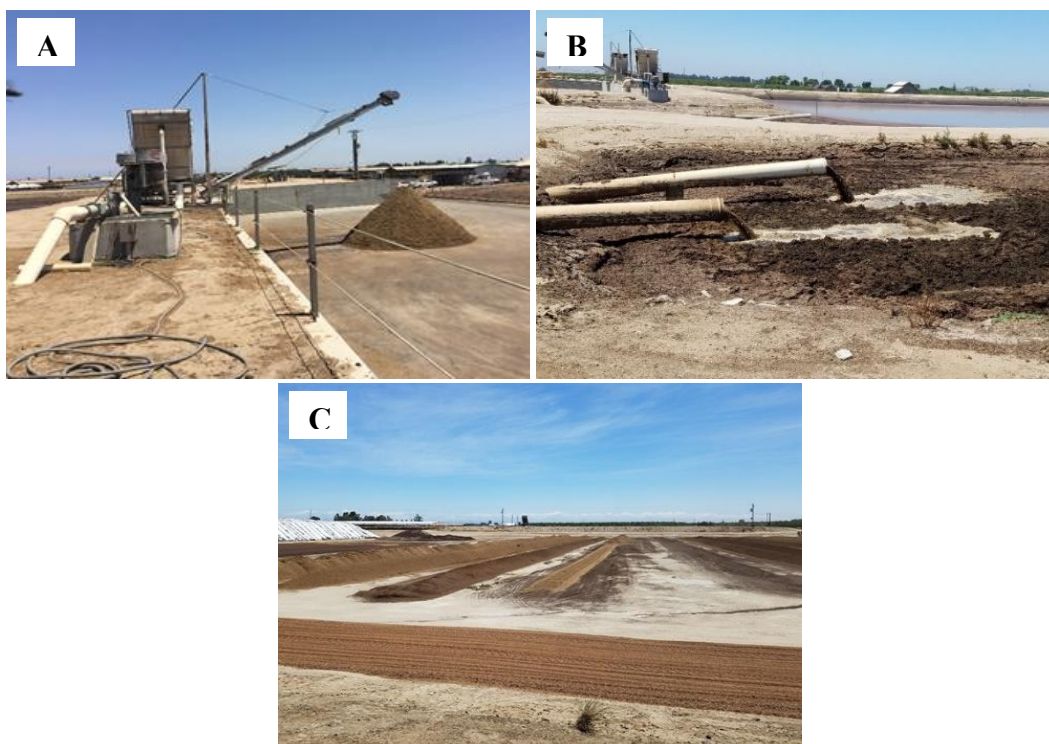
Figure 24. Dairy B: (A) coarse separator, (B) screened flush manure into sedimentation pond, and (C) windrow piles
