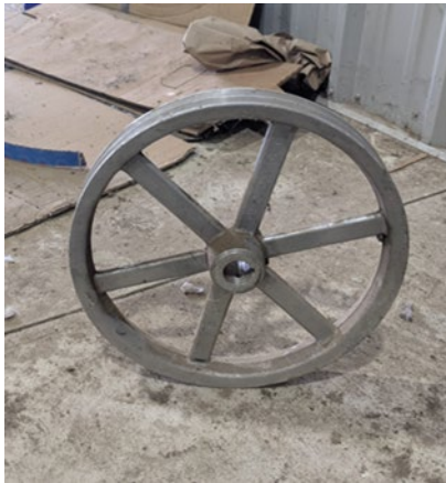
Pulley wheel for the Pellet Mill System Feed Auger.
