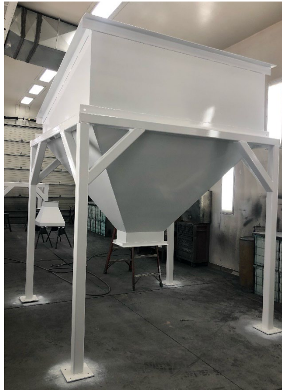
Components of the pelletizer system on the farm. Pictures include the hoppers, stands, compost surge bin, and augers for the pelletizer system in the warehouse in Wisconsin.
