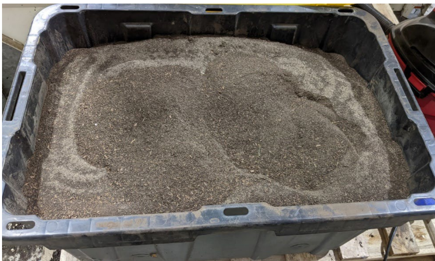
Full Scale Pellet Mill Testing at California Dairy Farms - Batch #2 Drier, sandier manure compost.
