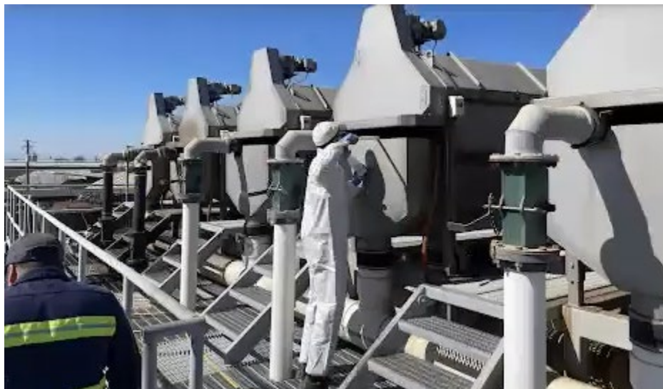
Sampling the inlet of the rotary drum separator.
