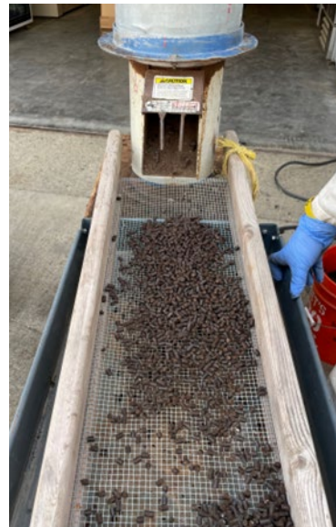
Small Scale Pellet Mill Moisture Testing. Ian and Hossein Pelletizing Manure Compost (left) and screened pellets (right).
