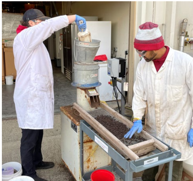
Small Scale Pellet Mill Moisture Testing. Ian and Hossein Pelletizing Manure Compost (left) and screened pellets (right).
