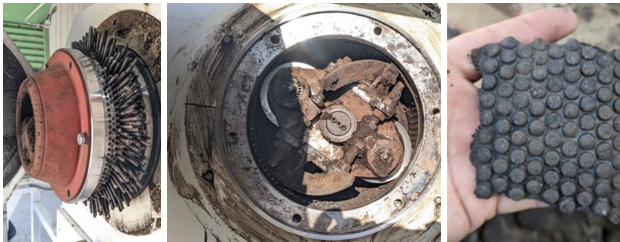
Full Scale Pellet Mill Testing at California Dairy Farms - (Left) Exterior of the Pellet Mill feed cone and die with pellets sticking out; (Center) Rollers and Die visible from inside the feed cone; (Right) Compressed composted manure removed from the feed cone after plugging of the die.
