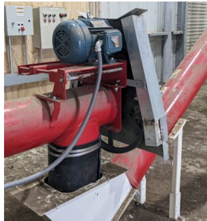
Pulley wheel for the Pellet Mill System Feed Auger.
