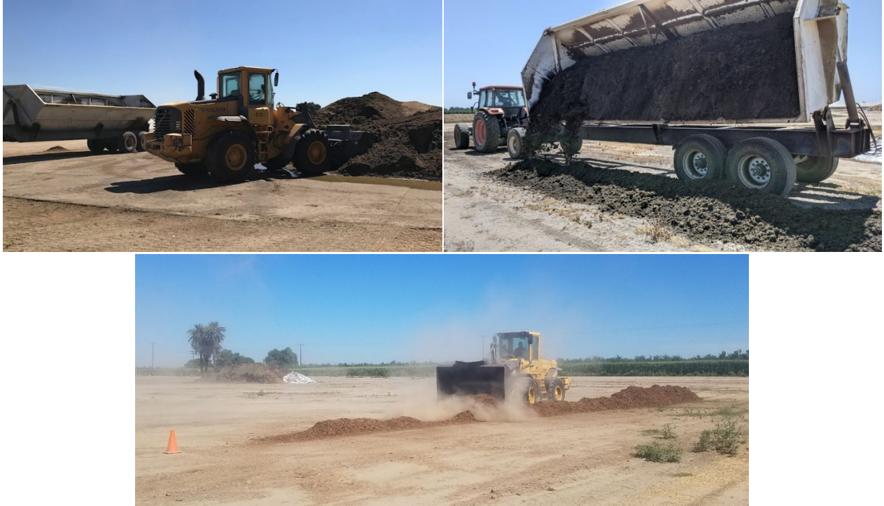
Constructing compost windrows: Top left and bottom photo taken for Healthy Soils Project but used to depict construction of compost piles. Top right photo shows centrifuge solids being dumped for windrow construction.
