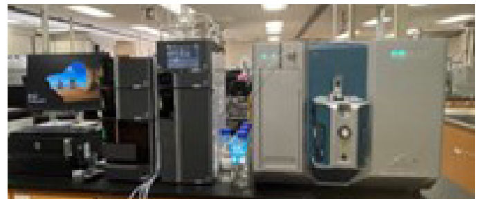
A new Sciex 7500 LC MS/MS in the CAC Environmental Safety Laboratory enhances inspection sensitivity by up to 10 times.
