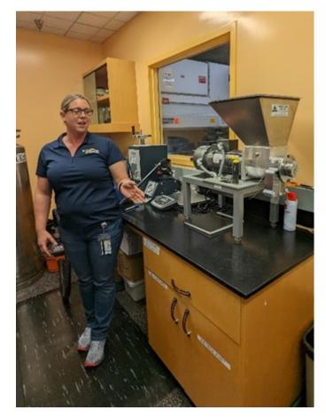
Sabine Hargrave shows equipment used to grind feed samples at the CAHFS Laboratory.
