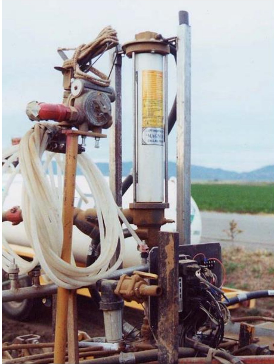
Figure 10. Anhydrous cooling tower and electronic module for controlling pulsed emissions.
