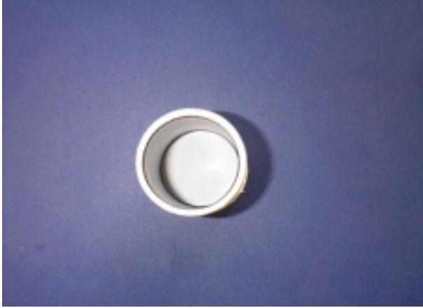
Photo 6. Aluminum sleeve glued with the filter paper (from the top).
