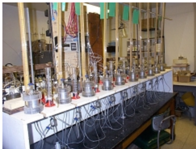
Photo 12. Multi-step experiment set up for the ten 2" Tempe cells.
