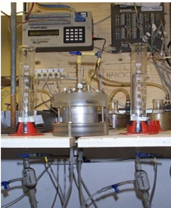
Photo 11. The 2" Tempe cell set up.
