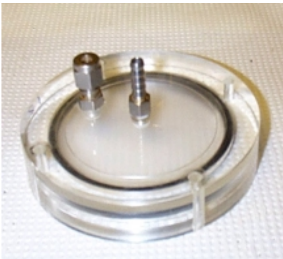
Photo 4. The 3.5" top cover of the Tempe cell.
