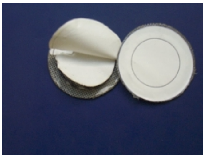
Photo 10. Porous membrane assembly and support.
