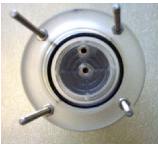
Photo 9. Bottom cover of the 2" Tempe cell.
