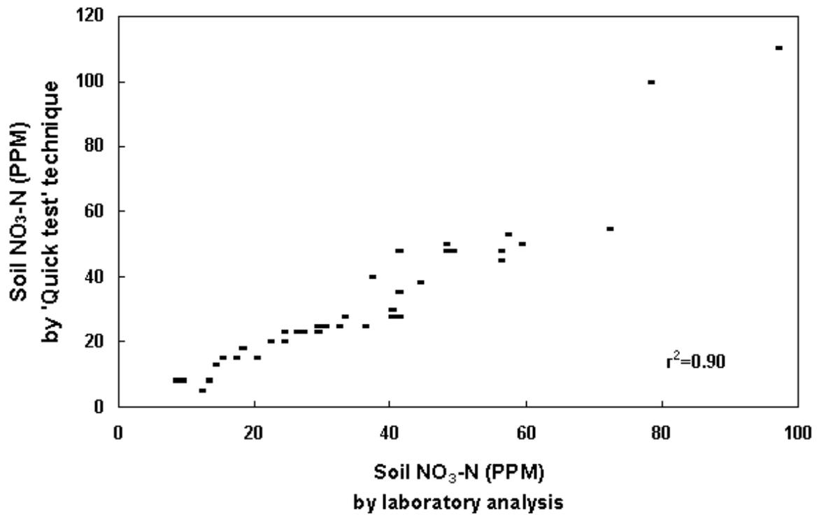
Fig. 1. Correlation of the soil 'quick test' techniques with conventional laboratory analysis of soil NO<sub>3</sub>-N concentration.
