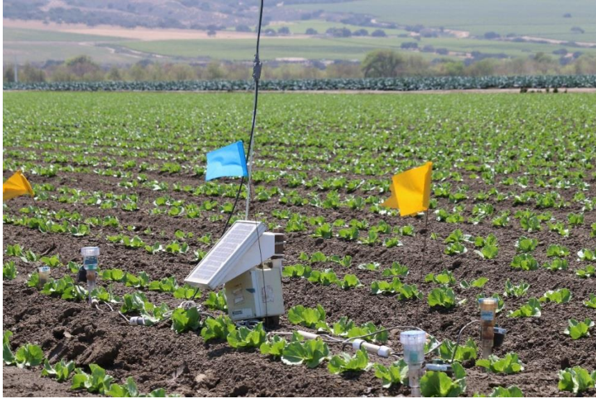
Figure 10. Tensiometers readings were automatically recorded to a datalogger and uploaded to CropManage through radio and cell phone communications.
