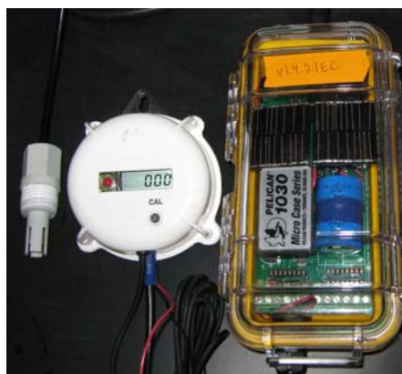
Figure 4. Electrical conductivity probe, display, and wireless node used for measurement of dissolved fertilizer in fertigation water.
