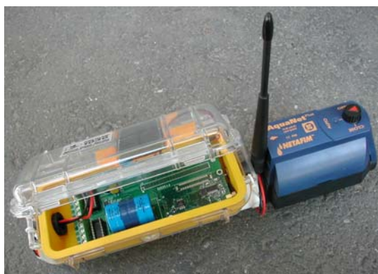
Figure 2. Wireless valve controller with 1-inch latching valve.
