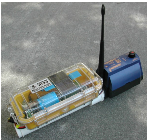
Figure 2. Third-generation valve controller with 1-inch latching valve.
