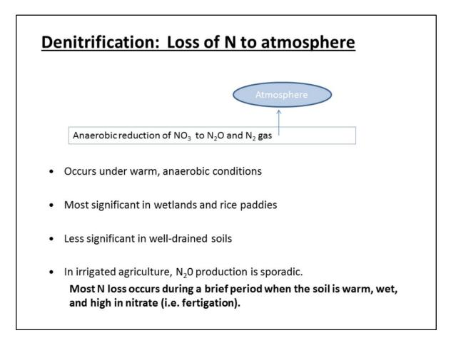
The chemical formula shows denitrification, the reduction of nitrate to nitric and nitrous oxide gasses, and dinitrogen gas, all of which can volatilize off the field. This conversion occurs in the presence of an available C source for anaerobic, heterotrophic bacteria that use the N in nitrate as an electron acceptor.(for energy)
