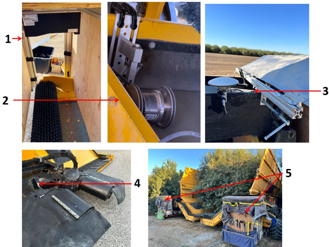
Figure 1: Almond yield monitoring system: 1. Laser profiler, 2. Wheel Encoder, 3. RTK-GPS, 4. Vibration sensor, 5. Enclosures to protect the laser projections
