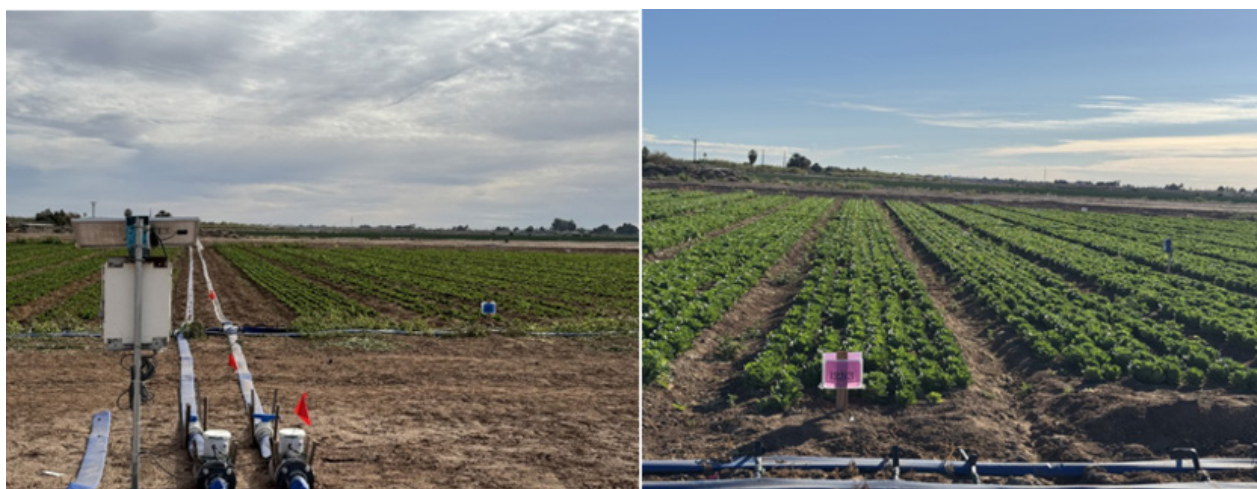
Figure 1. Little Gem lettuce field trial at the UC Desert Research and Extension Center during the 2025–26 growing season. Applied irrigation water was measured using magnetic flowmeters connected to a datalogger, with measurements automatically recorded and integrated into the CM platform for irrigation monitoring and management.
