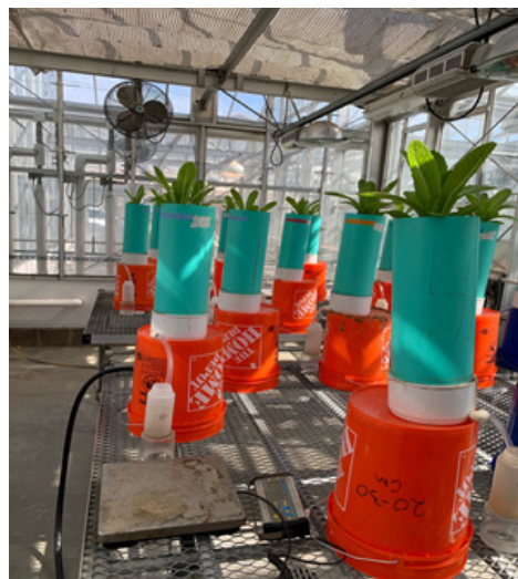
Figure 1. Experimental columns with lettuce, using a wide range of rates of compost addition to assess leaching of DON and inorganic N.
