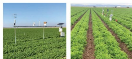
Figure 3. A fully automated ET tower is seen in the photo on the left. A multi-depths soil moisture sensor monitoring station equipped with Tule sensor is pictured on the right.
