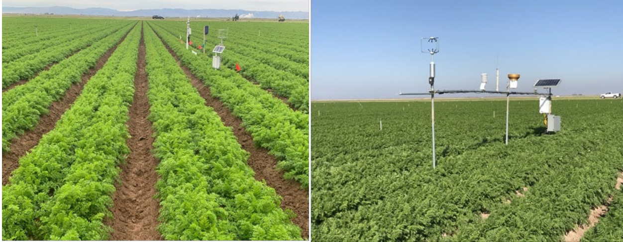
Fig. 2. Fully automated ET tower (right) and a multi depths soil moisture sensor monitoring station equipped along with Tule sensor in commercial sites (left).
