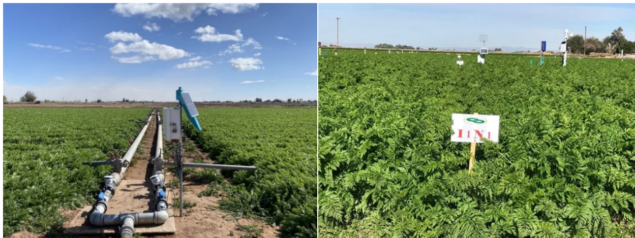
Fig.1. Magnetic flowmeters and data store and transfer equipment to monitor water applied to the trial (left) and monitoring station in treatment I1N1 at the UC DREC trial (right).
