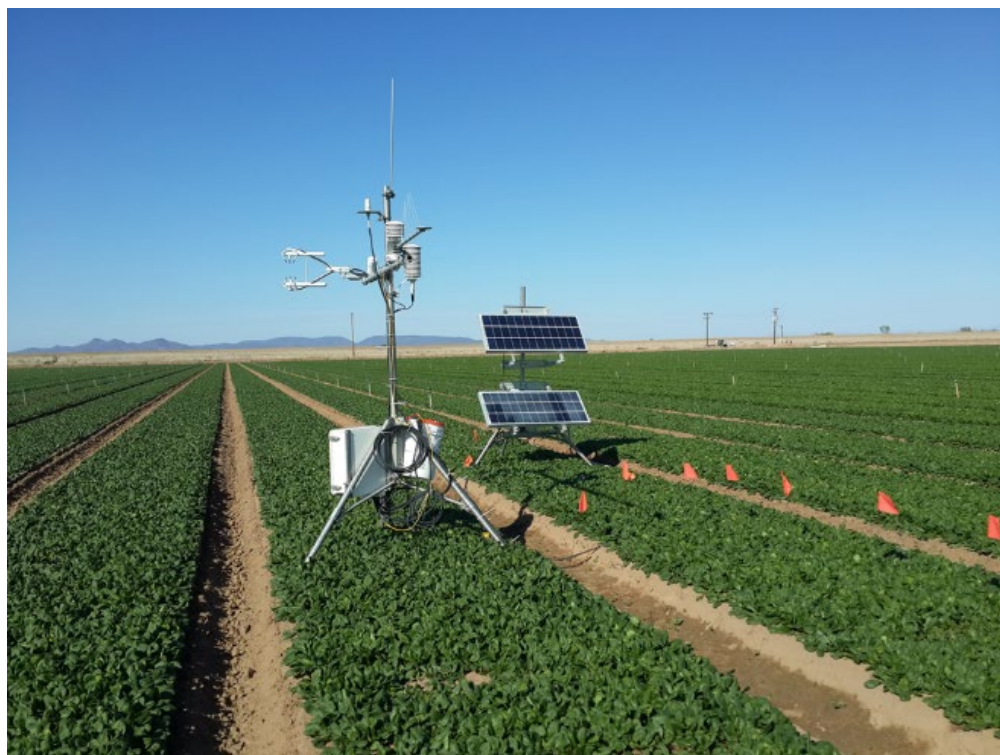
Figure 1. Typical eddy covariance set up in a baby spinach production field.
