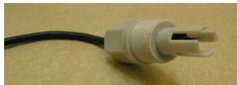
Figure 1. Electrical conductivity probe with threaded body for installation on fertigation line.
