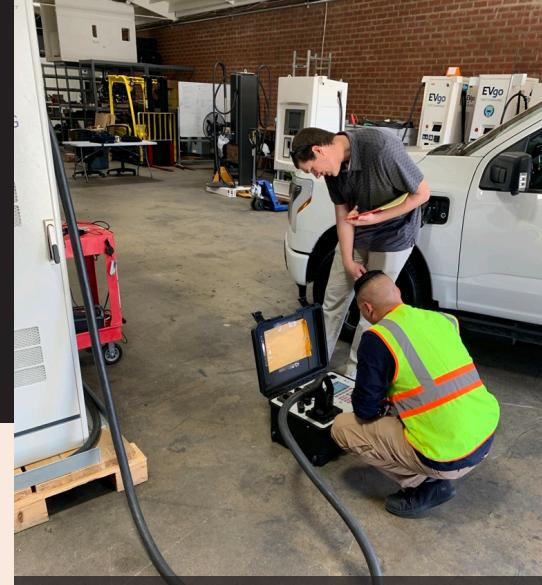
Type evaluation expert working with a Registered Service Agent to test new Electric Vehicle Supply Equipment (EVSE).
