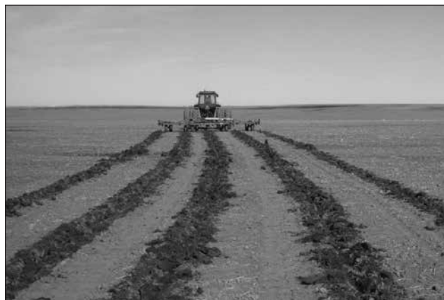
Figure 2. Tillage implement with very wide spaced shanks, making clods to roughen the soil surface. (Photo credit: John Smith, University of Nebraska).
