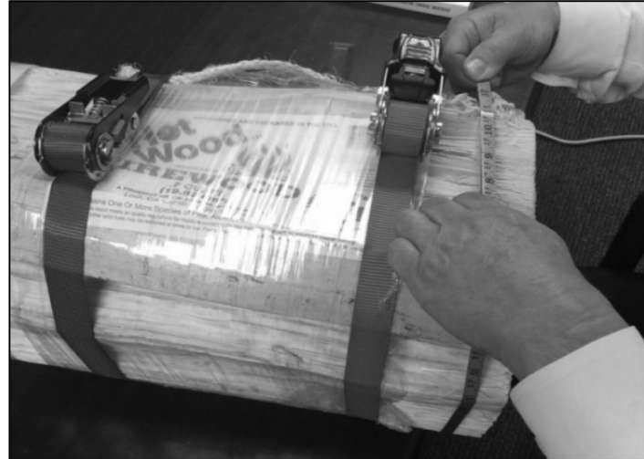
Figure 3-17. Strapping the Ends of a Bundle.
