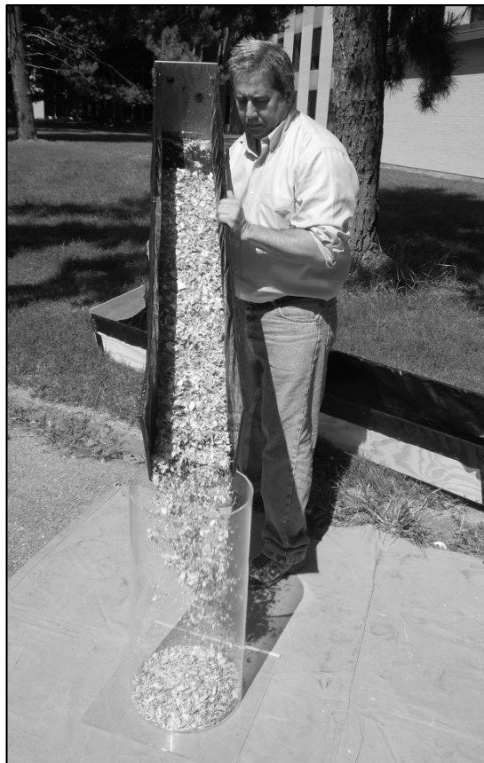
Figure 3-23. Filling a 44 L Test Measure.
