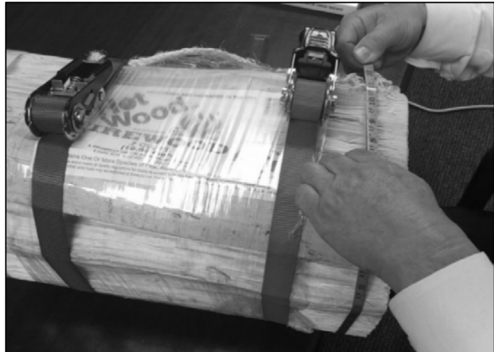
Figure 3-17. Strapping the Ends of a Bundle.
