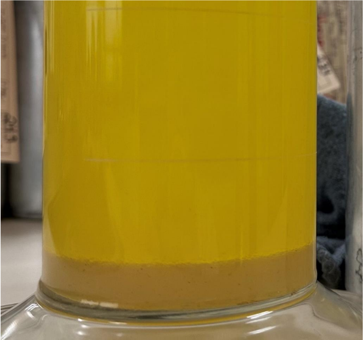
Figure 3: Diesel sample that is hazy (top layer) and contains water (bottom layer) as viewed from the side of the container.
