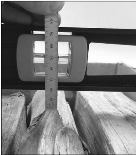
Figure 3-9a. Examples of the Headspace Measurement.
