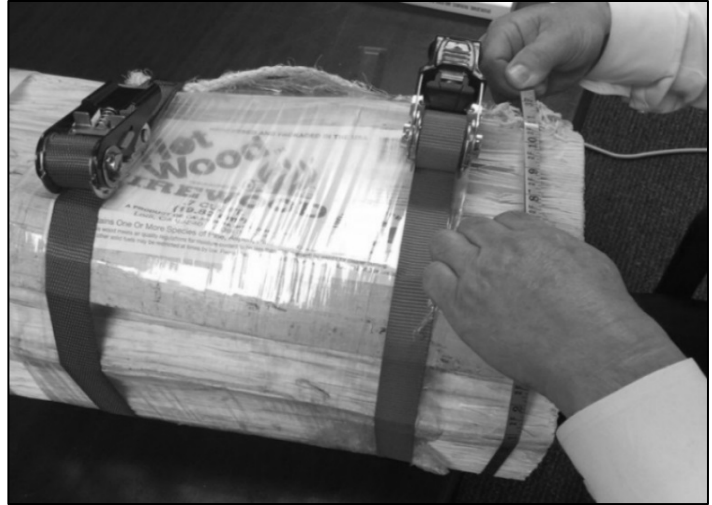
Figure 3-17. Strapping the Ends of a Bundle.
