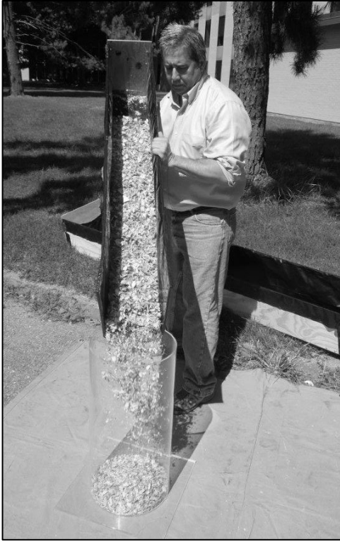
Figure 3-23. Filling a 44 L Test Measure.
