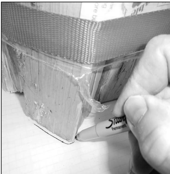
Figures 3-15. Tracing the Perimeter of the Wood.
