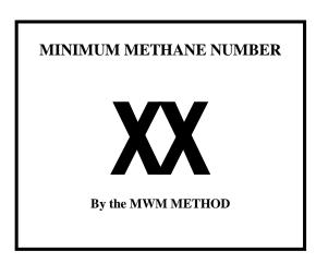
(c) All dispensers of natural gas motor vehicle fuel shall be labeled in a conspicuous place on each customer side "MINIMUM PERCENT METHANE XX" where XX is the minimum volume percent methane of the fuel dispensed expressed in a number rounded down to the nearest whole number. The label shall be a minimum size of 2.5 x 3 inches. The lettering shall be in Helvetica or Arial Bold font type, centered, in all capitals, and no less than 1/8 inch (0.32 cm) height.
