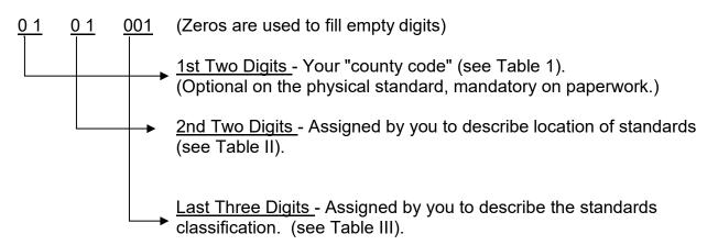
Standards which have identical descriptions, values and/or dimensional characteristics will have sequentially assigned 3-digit numbers. Example: Alameda County may have 4 each 50 lb. cast iron block office standards. The full serial numbers assigned to these standards could be: 01-01-001
