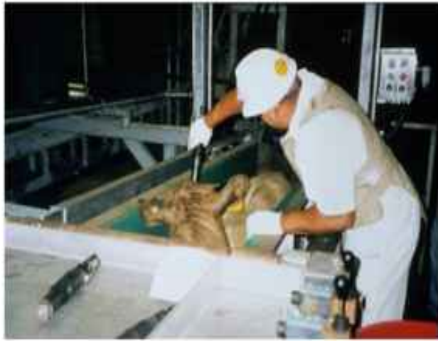
Captive bolt stunning in center track restrainer
