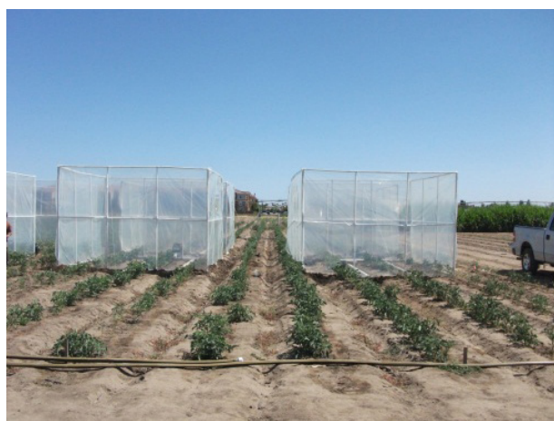
Figure 4. Photos of the open top chambers in which tomatoes were subjected to elevated CO_2 levels.
