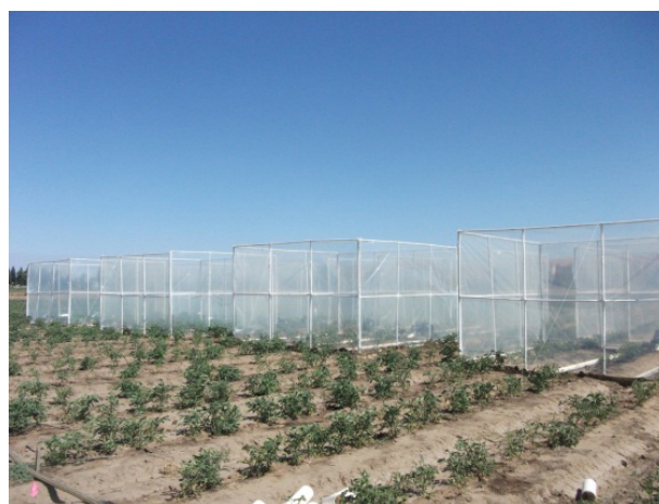
Figure 4. Photos of the open top chambers in which tomatoes were subjected to elevated CO_2 levels.
