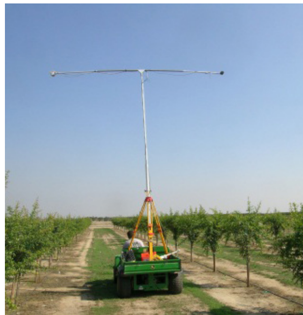
Figure 4. Pomegranate Canopy Cover measurements with a Multi-spectral Camera
