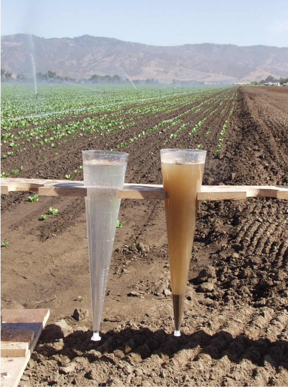
Figure 8. Tail-water run-off sampled from a sprinkler-irrigated lettuce field with (left) and without (right) polyacrylamide injected into the irrigation water at a 5 ppm concentration.
