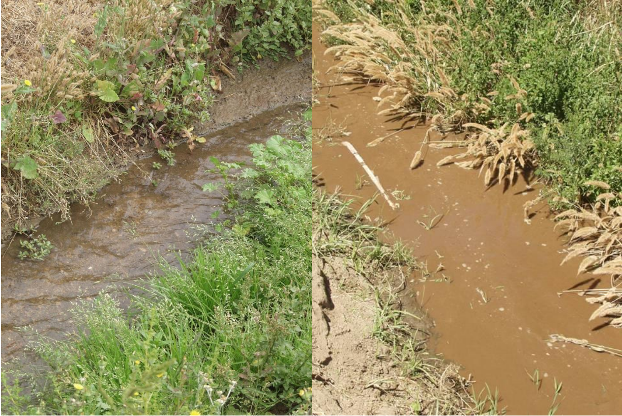
Figure 7. Run-off from a sprinkler-irrigated lettuce field with (left) and without (right) the injection of polyacrylamide in the irrigation water at a 5 ppm concentration.
