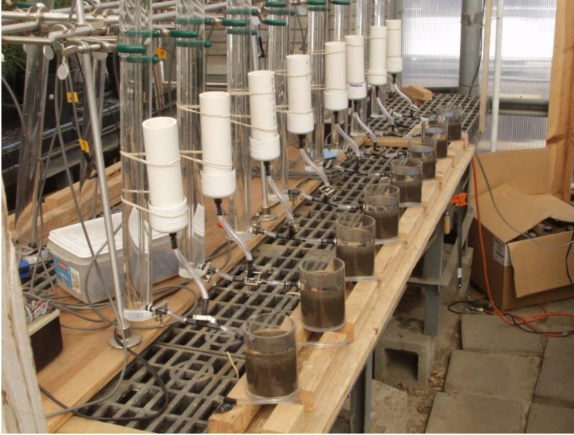
Figure 1. Columns and constant head burettes for measuring the effects of PAM on infiltration rate in a Salinas Clay soil.
