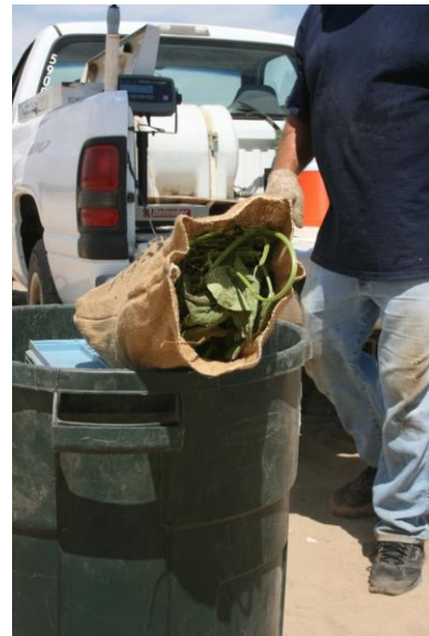
Figures 5 (left) and 6 (right). Canopy nutrient use estimates were made at the end of the season by weighing the vine from a 35ft 2 section of the plot, then taking a 1 lb sub-sample for nutrient analysis.
