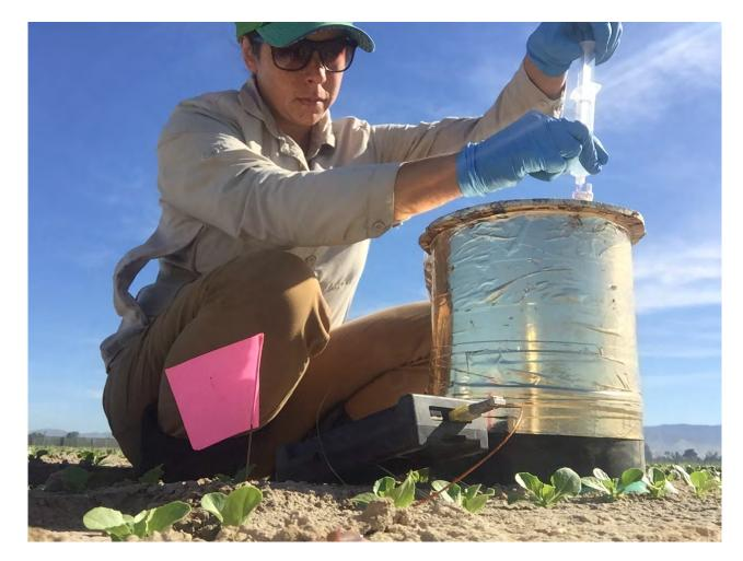
Samples of gas are collected from a septum in the chamber using a needle and syringe and brought to the lab for analysis on the Gas Chromatograph
