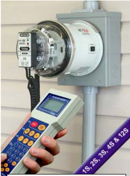
Probewell Standard with a mechanical rotation disk meter
