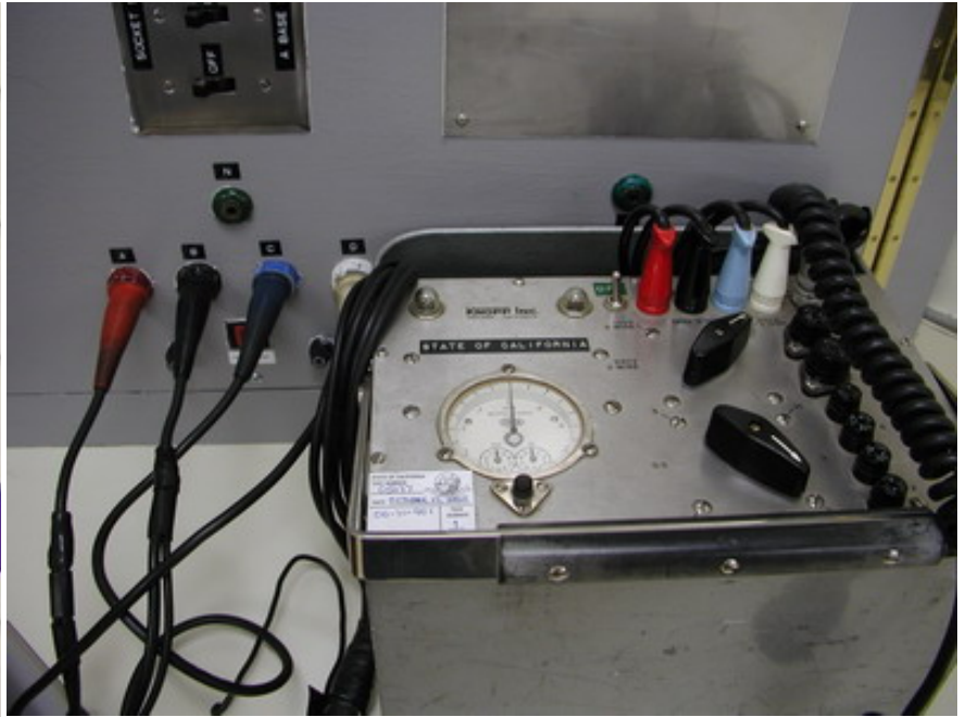
Knopp FS-8 Standard connected to a laboratory test board
