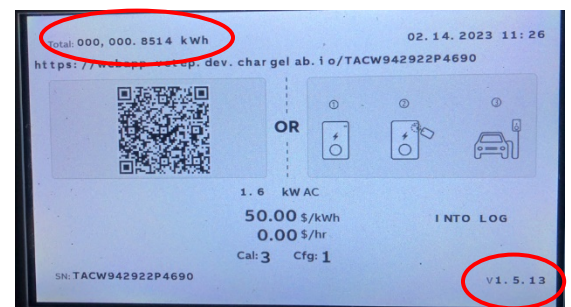
Figure 2. Totalizer and software version locations on the Terra EVFS screen
