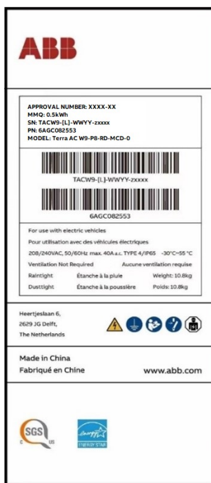
Figure 1. Sample ID label and its location on the side of the Terra EVFS
