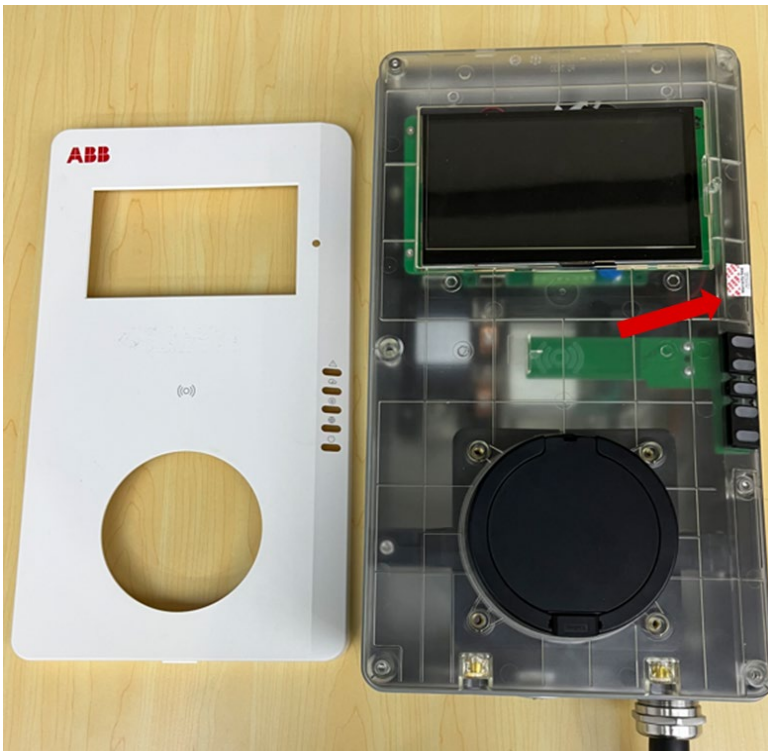
Figure 3. Location of the tamper evident security seal on the interior cover
