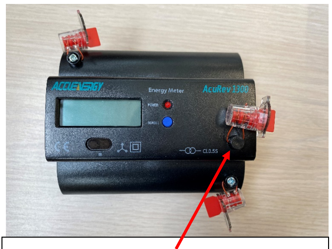
Figure 5. Wire terminal block sealing provisions with red arrow indicating the calibration button location
