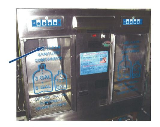
The ID badge is located on the wall of the fill area, to the right rear of the fill spout area.
