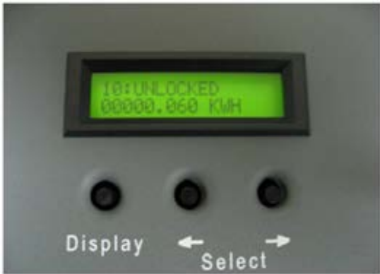
Figure 6. The “UNLOCKED” message should be visible on the LCD display and the unit cannot be used for commercial transactions.
