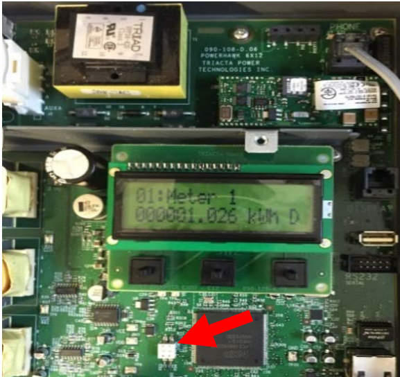
Figure 4. The red arrow points to the calibration DIP switch located on the main PCB. There are two switches in this assembly. When the meter is in service and sealed, both switches must be set to “off.” If the switches are set to “on”, then it is not sealed.
