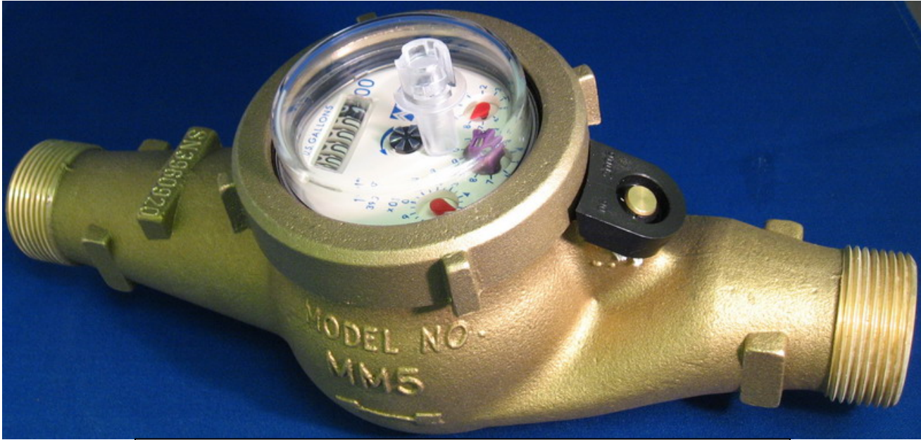
Fig. 1 Model MM5 showing serial number with SN preceding the serial number and Model NO. preceding the model number.
