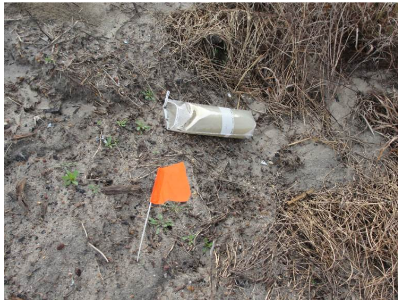
Figure 12. Pinned sterile 2 L Whirl-Pak® sample bags at Pond 1 prior to and after a runoff event.
