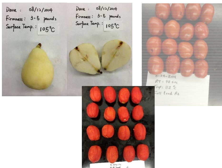
Figure 9. Peeled pears and tomatoes at temperatures of 105 and 112°C using IR peeling system.
