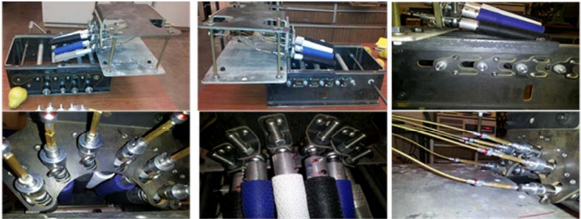
Figure 3 Elements of the fabricated prototype peel remover. The spring loaded fingers are equipped with special abrasive material to enable peel removal.
