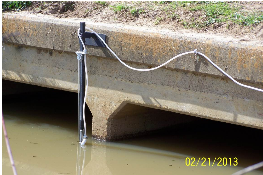
Figure 14. In the top photograph, Mr. Rodney Hill and Ms. Casey Harris install sterile Tygon tubing for the ISCO sampler at Pond 1 prior to a precipitation event. The bottom photograph shows the sampler intake installed just above base flow. The vertical position of the intake is easily adjusted.
