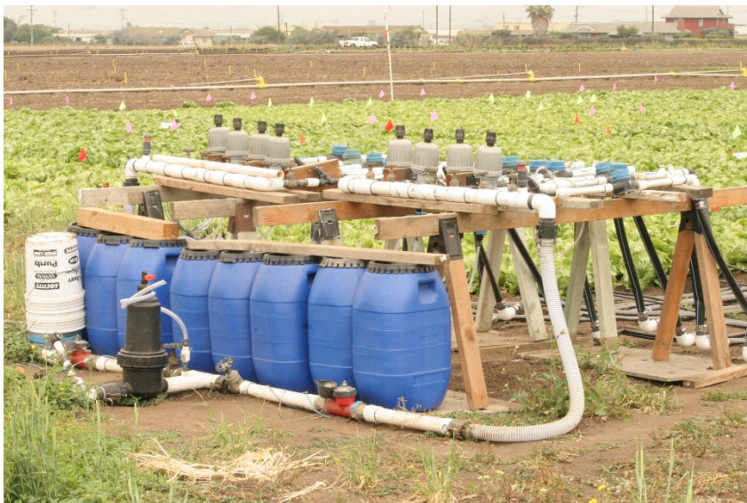
Figure 1. Manifold and injection system used for simulating irrigation water with different concentrations of nitrate-N.
